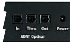
The Optical Thru port simply transmits a copy of the optical input data. By connecting the Optical Thru port to an ADAT machine, you can archive 8 tracks of audio to ADAT tape without recabling. Since the Optical Thru port acts as a repeater, you can also use it to send digital audio data twice as far as a single optical cable can reach.
